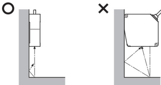
The detection surface (the side of the emitting/receiving parts) should be parallel to the target object. Adjust the spot to conform to the detection point. Ensure that the distance indicator turns orange when the detection point (the center of displacement) passes the spot point.
