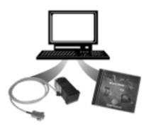
**N.B.**: RS232 interface for PC configurationè fornito is supplied with WINSTRUM programming software. make the connection with the device powered and with inputs and outputs disconnected.
