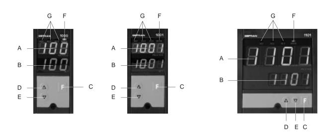
A - Digit height 14mm (1000), 10mm (1001), 20mm (1101) green Value of variable controlled to 3 digits (1000) 3<sup>1/2</sup> digits (1001 -1101) Indication - 199...+999 (1000) indication -999...+1999 (1001-1101) with decimal point on appropriate scales. Positive (HI) or negative (LO) off-scale message Message for broken/incorrect connection of probe; (SBR: open circuit / ERR: probe reversed) and display of configuration and calibration messages.
